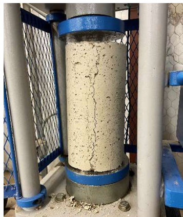
Figure 3. Students conducting compressive strength test.
