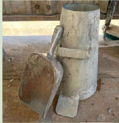
Slump Cone Test
