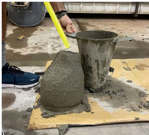
Figure 2. Students conducting slump cone test.
